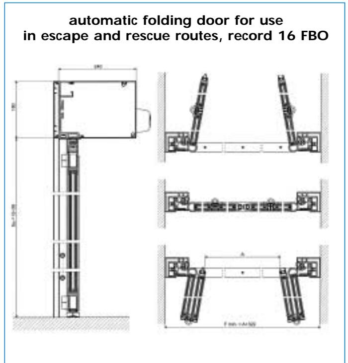
**A** : clear opening width    **G** : height of passage    **F** : length of operator header
